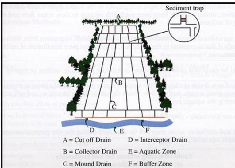
**Figure F: Schematic of Typical Forestry Drainage Layout**
